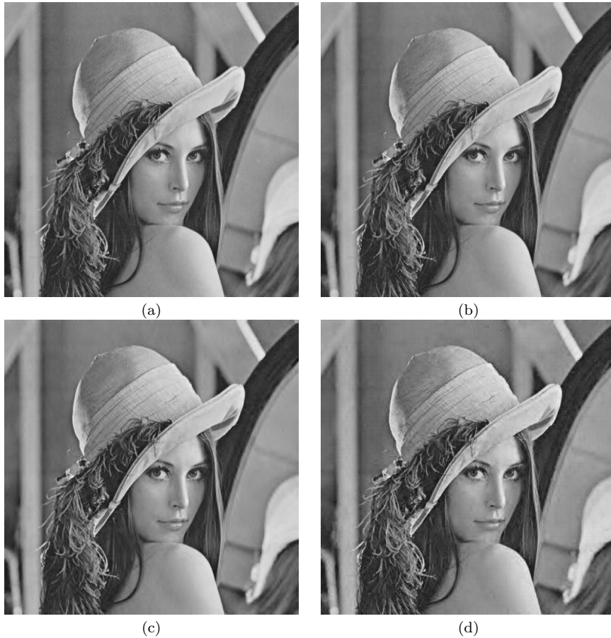
Fig. 8 Lena image watermarked and compressed with our joint scheme at 1.6 bpp with different step size values: (a) \Delta_{TCQ} = \Delta/4 (PSNR = 43.09 dB, SSIM = 0.9658), (b) \Delta_{TCQ} = \Delta/2 (PSNR = 41.86 dB, SSIM = 0.96021), (c) Watermarking and JPEG2000 compression with \Delta_{TCQ} = \Delta (PSNR = 39.53 dB, SSIM = 0.9412), (d) Watermarking and JPEG2000 compression with \Delta_{TCQ} = 2\Delta (PSNR = 36.28 dB, SSIM = 0.9010).
