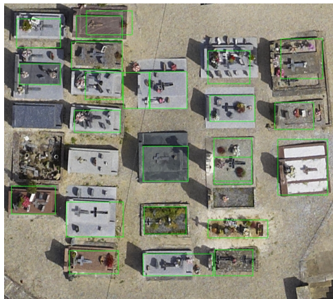
Figure : Results obtained on an aerial view of a part of Lecey cemetery. Green rectangles represent the bounding boxes of the detected tombs.
