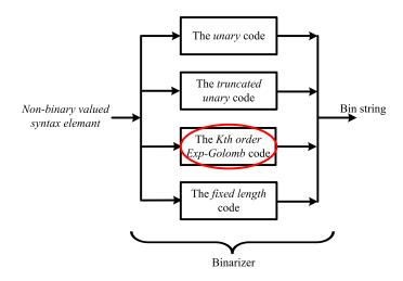
Figure 3: Block diagram of binarization stage illustrating different binarizatin methods.
