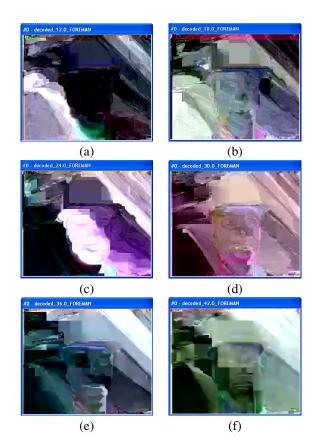
Figure 6: Decoding of encrypted video "foreman": first frame with QP equal to (a) 12 (b) 18 (c) 24 (d) 30 (e) 36 (f) 42.
