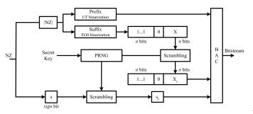
Fig. 4. Encryption of NZs in CABAC of H.264/AVC.
