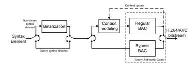
Fig. 2. Block diagram of CABAC of H.264/AVC.
