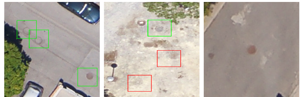
Figure 5. Examples of detected manholes covers, false positives and non detected manhole covers by the customized network. Green boxes correspond to detected manholes covers, red boxes to false positives.
