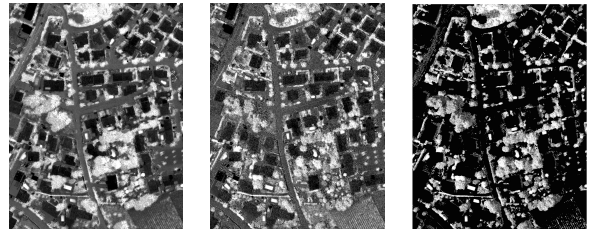
Fig. 4. Detection of vegetation using, left: NDVI, middle: ExG and right: fusion of the two previous results. Whiter pixels belong to the vegetation class.
