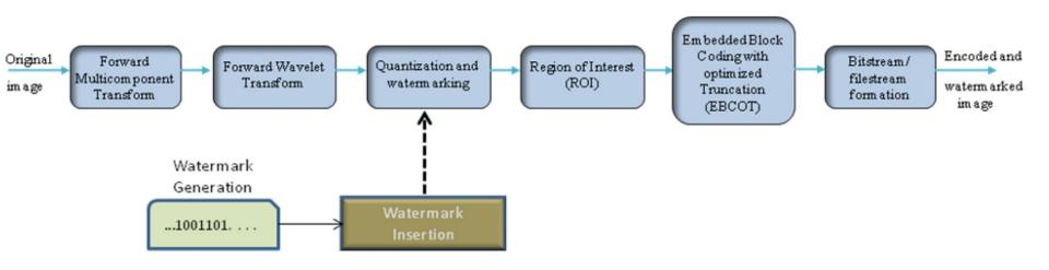
The joint JPEG2000 encoder/watermark embedding scheme.
