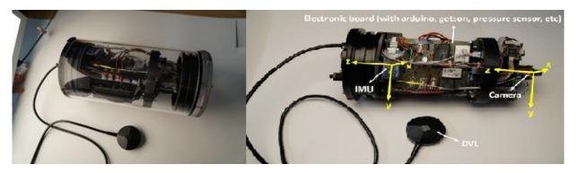
The waterproof underwater capsule of the smart camera system (left) and the smart camera system description with reference frames fixed to it (right)
