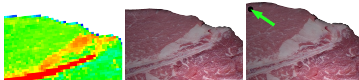
Fig. 1.11: The flesh and the fat, although interpolated between the same two control frames, pulled at the black point, exhibit different strains due to different stiffnesses.
