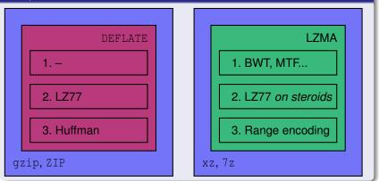
LZ77 coding Canonical Huffman coding Flow control with blocks
