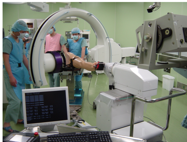
▲ Robot to assist femur fracture reduction
