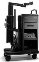
Aesop, camera-holding robot for laparoscopy, voice controlled (Computer Motion Inc., USA)
