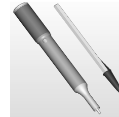
Active hand-held instrument for tremor compensation (CRIM Lab).
