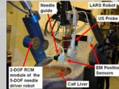
A Dual-Armed Robotic System for Intraoperative Ultrasound Guided Hepatic Ablative Therapy Boctor, Fitchinger, Taylor-ICRA 04
