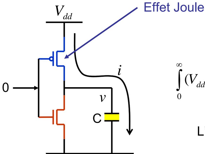
$$\int_0^{\infty} (V_{dd} - v) i dt = \int_0^{V_{dd}} C (V_{dd} - v) dv = \boxed{\frac{1}{2} C V_{dd}^2}$$
