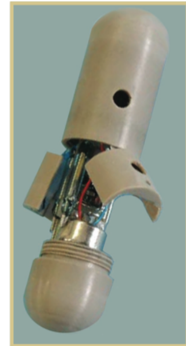
Figure 6. In the IDEAS (Integrated Diagnostics for Environmental and Analytical Systems) project's Laboratory in a Pill, a plastic shell encapsulates the device electronics. (image courtesy of the IDEAS team)
