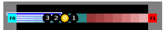
(a) Closest Frontier Allocation : all robots are assigned to the same, closest, frontier
