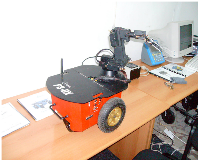
Fig.1: Mobile platform Pioneer 3-DX WMR.
