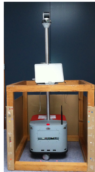
Figure 1: Testing Robot's Laser Rangefinder Inside a Box
