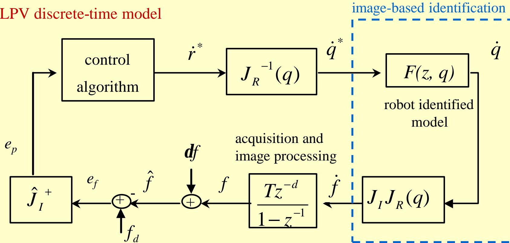
GPC of a 6DOF robot vision loop :
