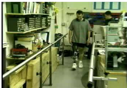
Speed & Patient Adaptive MagnetoRheological Knee Prosthesis (MIT, USA)
