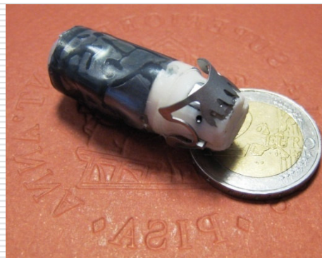
Wireless capsule based clip release
