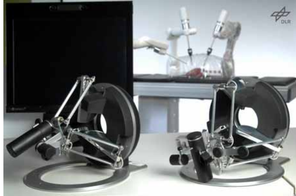
© DLR MiroSurge - a robotic system for research in minimally invasive surgery with haptic feedback
