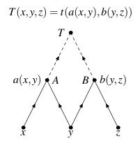
node A gets x and y and computes some function a(x, y); node B gets y and z and computes some function b(y, z); finally, the output node T gets a(x, y) and b(y, z) and should compute T(x, y, z).
