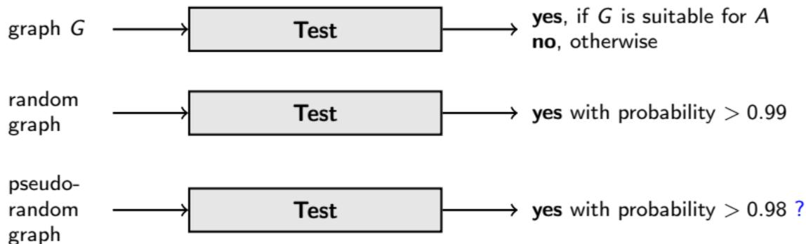
**Test** is an  $AC^0$ -circuit [size  $\text{poly}(m)$ , depth  $O(1)$ ].
