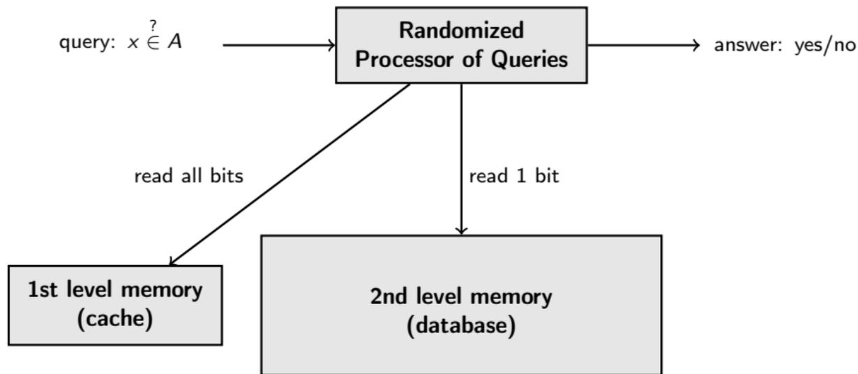
**Theorem.** For any  $n$ -element set  $A$  from an  $m$ -element universe there exists a randomized bit-probe scheme with one-sided error, with cache of size  $O(\log^c m)$  and database of size  $O(n \log^2 m)$ .
