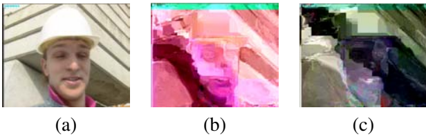
Fig. 19: Key sensitivity test for encrypted frame #1 of foreman video sequence for QP value 18. Encrypted frames are decrypted and decoded with: a) original key, b) 1-bit different key(SE-CAVLC), c) 1-bit different key(SE-CABAC).
