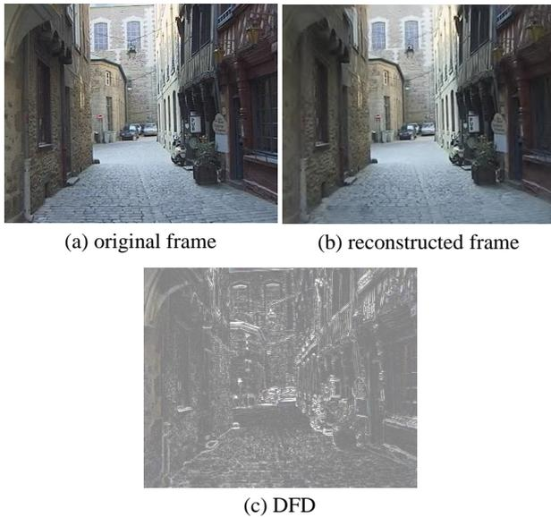
**Fig. 2.** Example of lossy motion coding for sequence Rue. While visual quality is good for reconstructed frame, DFD is large due to lossy coding of motion information. PSNR of reconstructed frame is 20dB.
