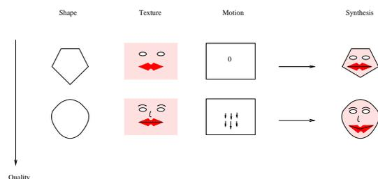
Fig. 1. Scalable video object coding based on progressive shape, texture and motion informations.
