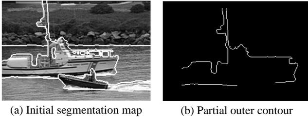
Fig. 4. Extraction of the apparent contour of an object
