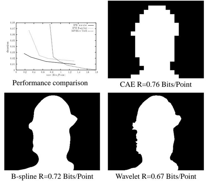
Fig. 6. Comparison of contour coding techniques. Average percentage of erroneous pixels with respect to average bit-rate per contour element. Sequence Foreman.
