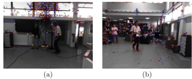
Fig. 15 (a) In this area localization is more difficult, mainly due to the lack of textured features. (b) Even though there are some persons walking in the environment occluding some visible 3D points, the algorithm is able to find correct pose estimates without problems. The red circles are the detected 2D features, the blue crosses represent the re-projection of predicted visible 3D points. The set of inliers putatives after solving the PnP problem are represented by cyan rectangles, whereas the outliers are represented as yellow rectangles. Best viewed in color.
