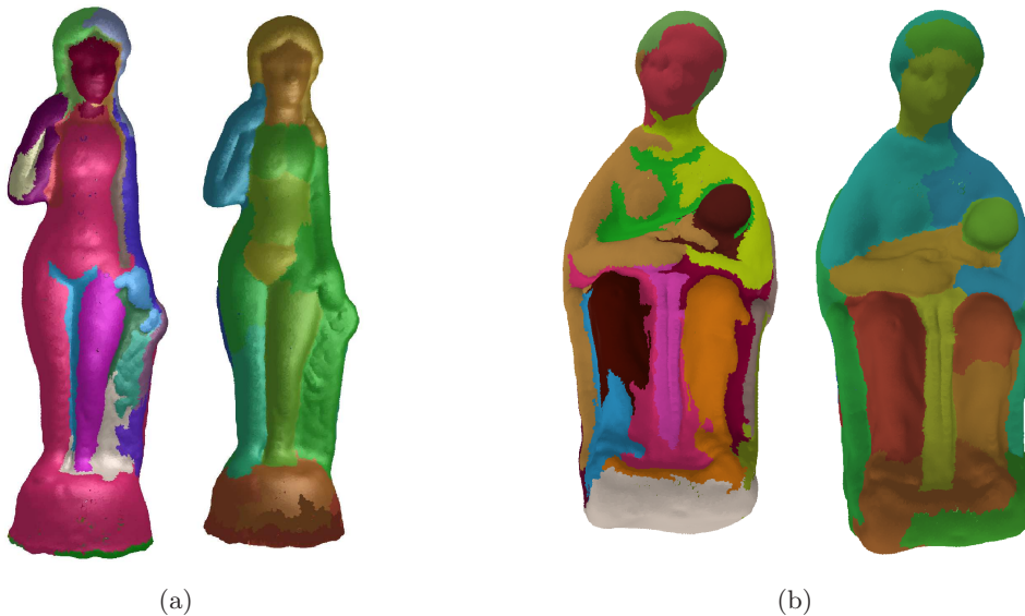
Figure 3.1: Perceptual grouping problem: the figurines [ED] were segmented using two different strategies, but both producing acceptable results and they mimic different human perception. The models on left were segmented using our MST-based algorithm [ADC07b] and the models on right were segmented using a watershed segmentation algorithm [APFJ + 08a].
