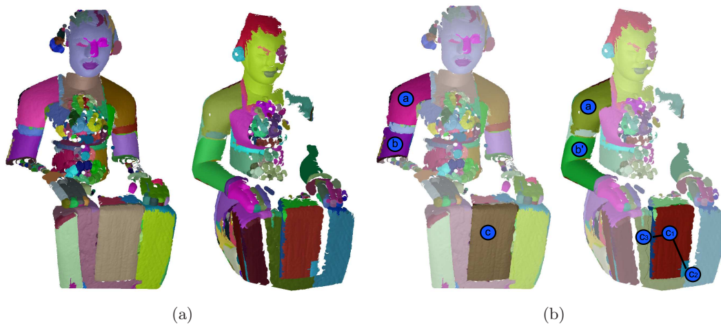
Figure 4.2: Equivalence condition. (a) Two scans represented by a region set. (b) Correspondence between regions when the region absolute property is taken as its shape, where we outline some regions for better illustration of the concept. Matched regions have the same region index.
