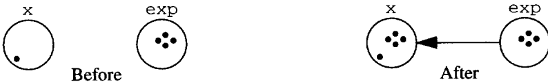
Fig. 2. The situation before and after establishing the constraint for x := \text{exp} and propagating.
