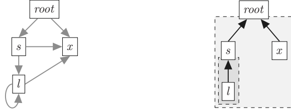
Fig. 4. Object graph (left) and ownership tree (right) for the example in Fig. 3. UT and OT give rise to the same ownership tree. In the object graph we show all references between objects. In the ownership tree we draw an arrow from the owned object to its owner and put all objects with the same owner into a dashed box.
