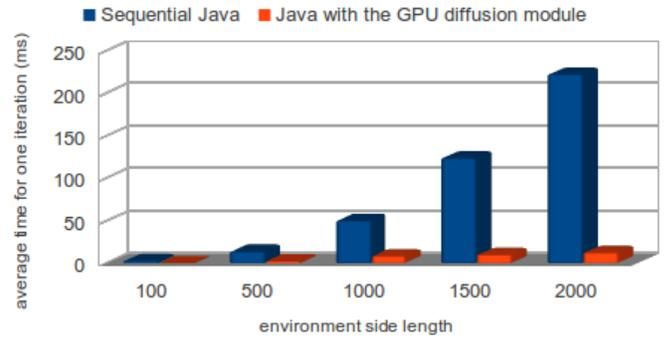
Fig. 2. Diffusion process: Java sequential vs. JCuda
