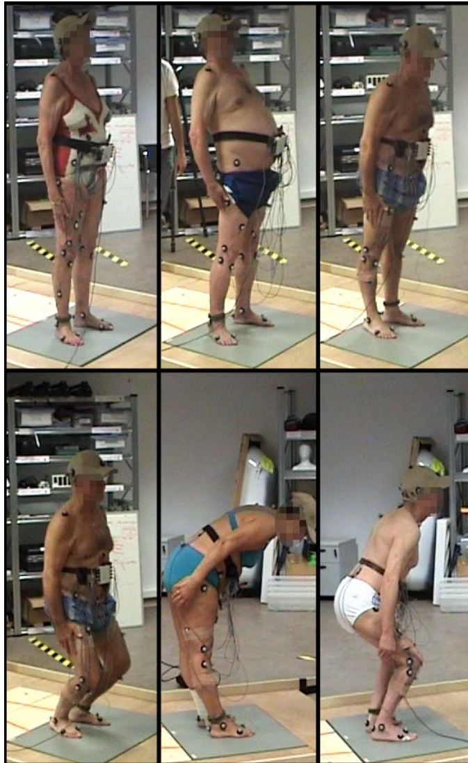
Figure 7. Six static poses required to identify the SESC locating the subject's CoM.
