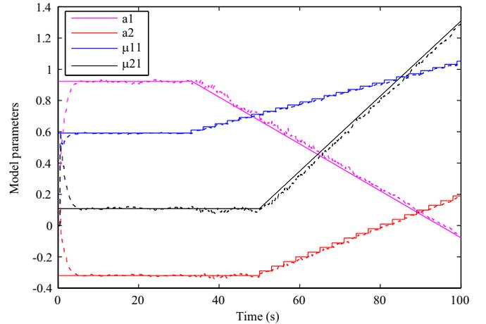
Fig. 10. Convergence and tracking of model parameter estimates for both static and time-variant parameters. Solid lines indicate true parameters. Dotted lines indicate parameter estimates. All the initial estimates were set at zero.
