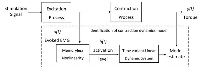
Fig. 4. Muscle model structure. The present work focuses on the contraction dynamics model contained in the rectangle within the dashed line. The memoryless nonlinearity is modeled by an  $n$ th-order polynomial function. The linear dynamics is chosen as an ARX model.
