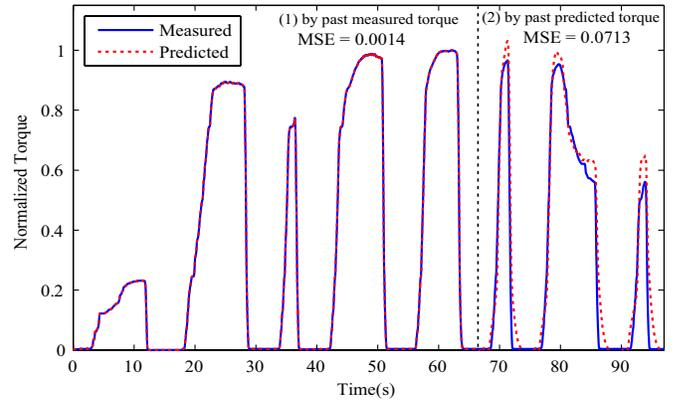
Fig. 7. The measured and predicted torque obtained by eEMG-to-torque model in random test. The vertical dotted line is shown to separate the data into two parts. (1) The torque was predicted based on the past measured eEMG and past measured torque. (2) The torque was predicted based on the past measured eEMG and past predicted torque, and the predicted torque was initialized at 0.
