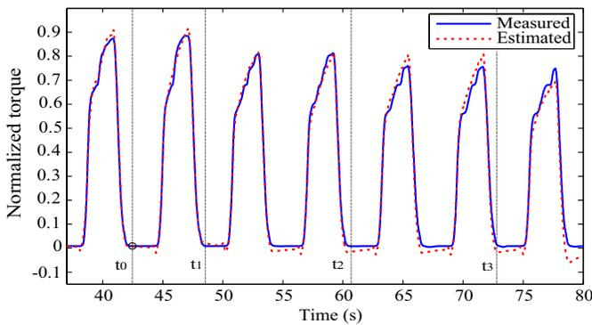
Fig. 12. Measured and estimated torque at time instant  $t_0$ . For evaluating prediction performance, the prediction errors for prediction horizons  $t_1$ ,  $t_2$ , and  $t_3$  (6s, 18s and 30s respectively) are measured. A KF with forgetting factor 0.997 was used to estimate the model.
