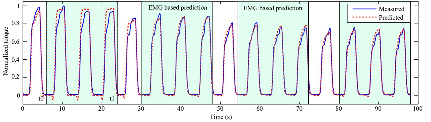
Fig. 14. Fatigue tracking based on eEMG-to-torque model and Kalman filter in subject S3. The model estimated at instant  $t_0$  was used to predict the torque from instant  $t_0$  to  $t_1$ , while the online identification and state estimation are switched off for 18s (with green background color). This process is repeated until the end of stimulation. The blue solid line indicates the measured torque, while the red dotted lines indicate the predicted torque.
