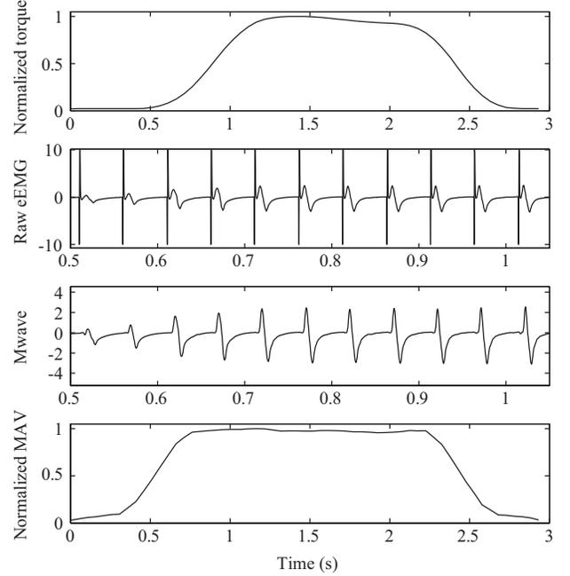
Fig. 3. An example of processed eEMG and torque. The raw eEMG signal and Mwave are zoomed in (0.5s ~ 1.1s) to show the details. The Mwave is overwhelmed by stimulation artifacts seen from the raw eEMG signal. Blanking window was applied to remove artifacts so that Mwave was effectively extracted.
