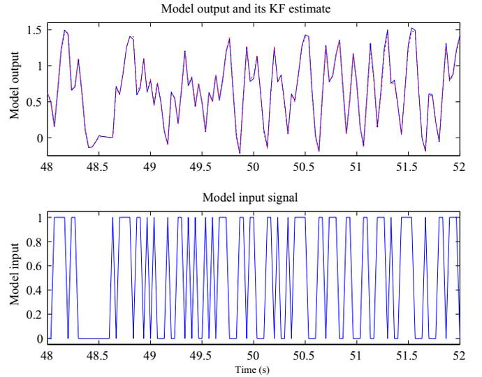
Fig. 9. Data set for model estimation. Data are generated by simulation using a PHM  $(2, 2, 1)$ . A KF with forgetting factor 0.97 was used to estimate the model.
