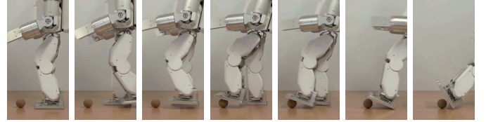
Fig. 9. A kicking motion planned for a ball at position x = 1\text{cm} and impact point h = 3\text{cm} , is used with a smaller ball that would have required a lower impact point, and which is at an unexpected position. The robot falls.
