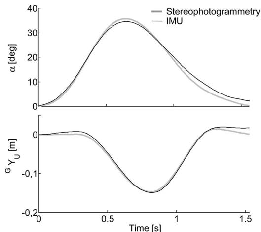
Fig. 7. Representative results showing the estimates of the IMU orientation  $\alpha$  and vertical displacement  ${}^G Y_U$  obtained for one randomly chosen subject. The corresponding RMSD were  $\alpha = 1.8^\circ$ ,  ${}^G Y_U = 7$  mm.
