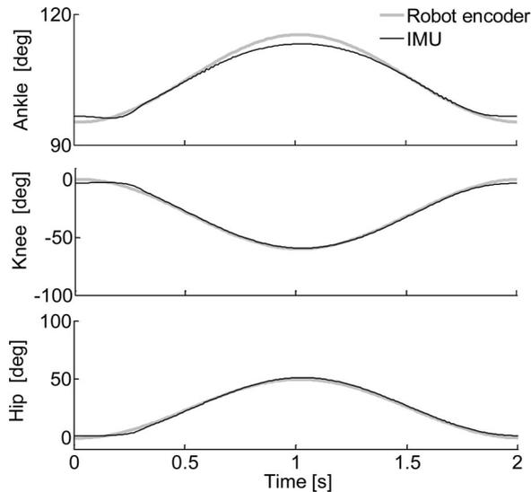
Fig. 6. Results obtained for the joint angles of interest in the squat task performed by the HOAP-3 humanoid robot.
