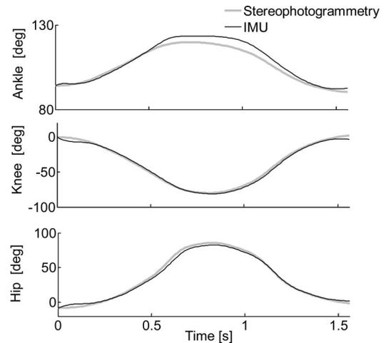
Fig. 8. Representative results showing the joint angles obtained for one randomly chosen subject. The corresponding RMSD were  $\theta_1 = 2.9^\circ$ ,  $\theta_2 = 2.2^\circ$ , and  $\theta_3 = 2.6^\circ$ .
