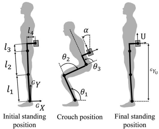
Fig. 2. 3-DOF biomechanical model of the human body. The point U represents the location of the IMU. The global frame  ${}^G X^G Y$  has its origin coinciding with the ankle joint centre and it is supposed to be stationary over the time.
