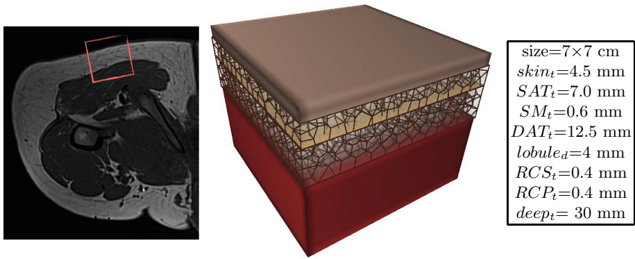
Fig. 2. SSC model for the buttocks based on parameters measured in a MR image
