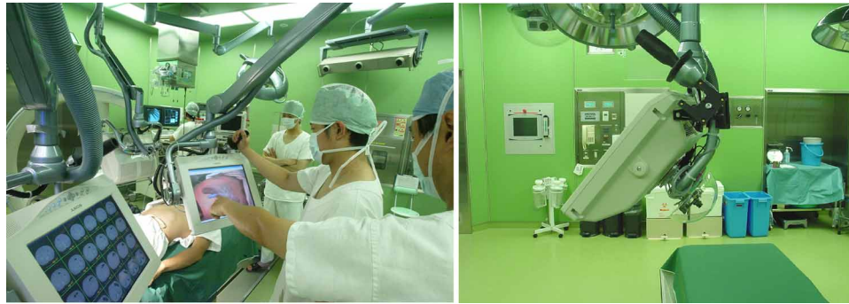
Figure 3. The setup of the data-fusion display. The operator is moving the monitor to the position from where he wishes to observe the inner structure. A small-size video camera is inset in the back of the monitor. [Color version available online.]
