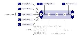
By pushing a label, we can create a higher hierarchy LSP (Label Switched Path), called **TUNNEL**.
