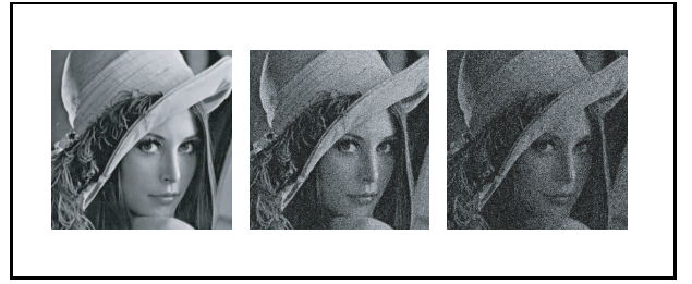
Figure 2: images of Lena with simulated Gaussian noise with standard deviations of 0, 30 and 60.
