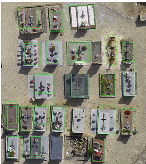
Fig. 6. Results obtained on an aerial view of a part of Lecey cemetery. Green rectangles represent the bounding boxes of the detected tombs.
