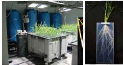
Left: the growth chamber is composed of hydroponic tanks where are immersed two-dimensional hydroponic-based boxes called rhizoboxes. Right: color image of a rhizobox and its mature rice root system.
