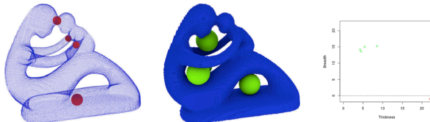
Figure 2.17. Fertility : there are five, and not four 1-holes. The most fragile parts of the object are represented by the thickness balls in the arms and between the heads. The thickness ball in the base is more difficult to appreciate, as the hole formed by the legs does not have a tubular shape. For a color version of this figure, see www.iste.co.uk/mari/analysis.zip
