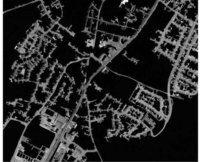
Fig. 3. Roads detection using gray-level threshold and extraction of the biggest connected components.
