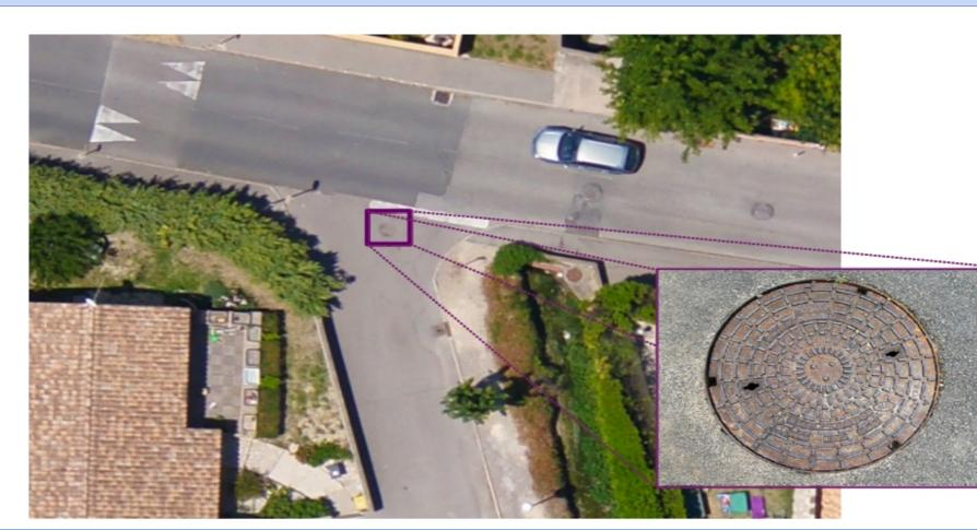
We propose to automatically detect manhole covers from aerial images in order to rebuild the network.
