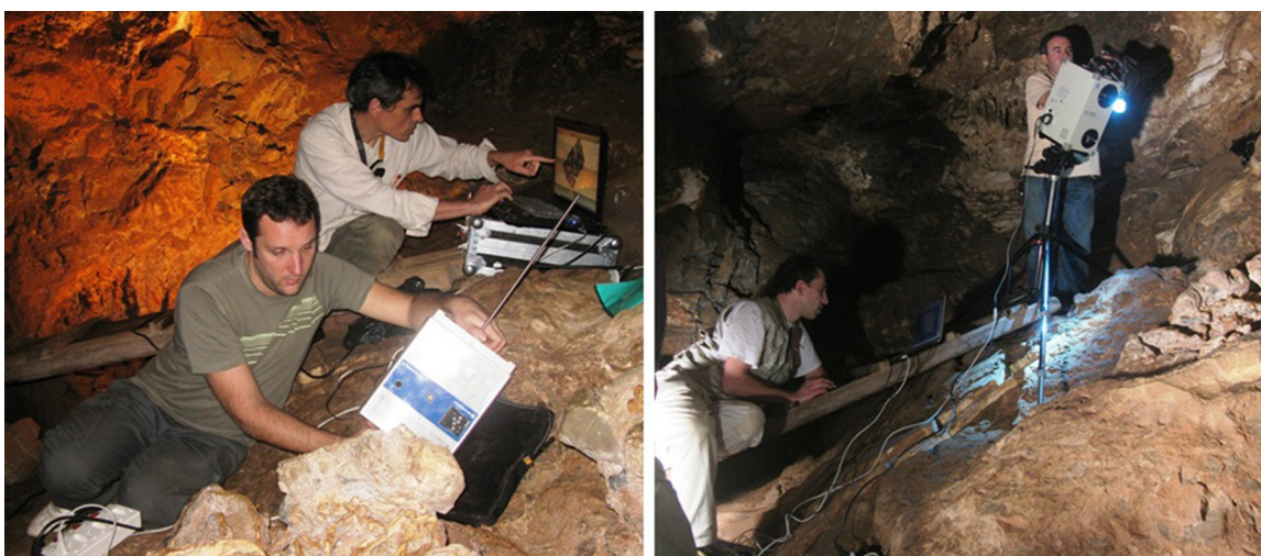
Figure 3. The 3D digitizers in situ: left the NextEngine HD; right: the Minolta VIVID 910.
