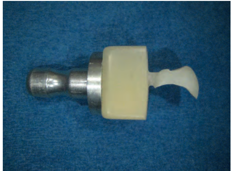
Fig.9: Crown milled in VITA ENAMIC block.
