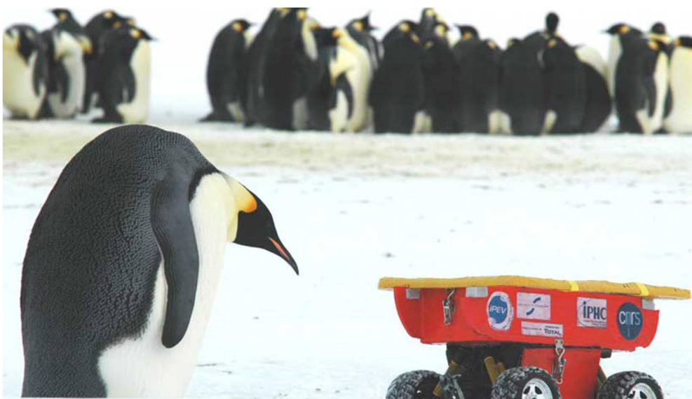
Figure 4. UGV deployed at Dumont D'Urville, Adélie Land, Antarctica to perform observations of breeding Emperor penguins ( Aptenodytes forsteri ). Courtesy Yvon Le Maho.
