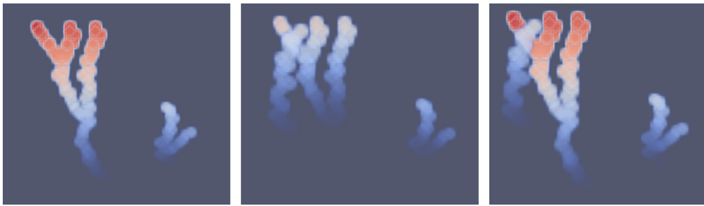
Fig. 7. On the left we can see the plot of the constrained distance function D^1 , in the middle we can see the plot of the constrained distance function D^l , l > 1 and on the right we can see the plot of the combined distance function D after time step l . Information about the (most left) simply connected component of the 4D segmentation which was not detected in the 1st time step is added into the function D in time step l . The values of D in the previously detected simply connected components were not changed by values of D^l .
