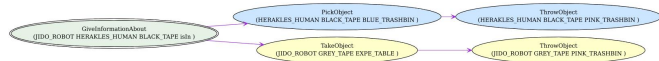
Figure 6. Plan produced for the first scenario. The robot informs the human about the location of the grey tape.
