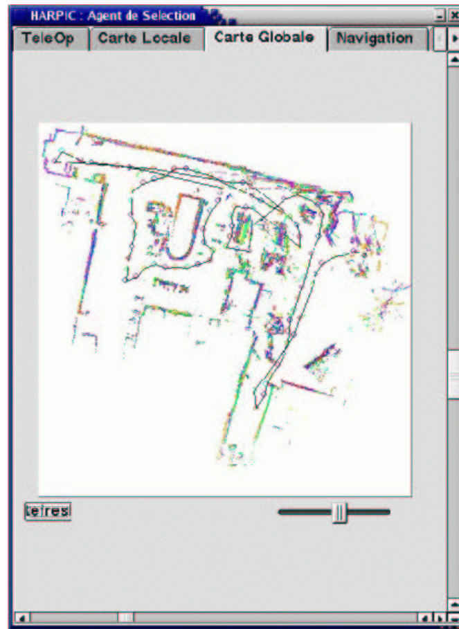
Figure 8. Map and robot trajectory generated during a JNRR'03 demonstration in the IFMA hall. Each circle on the robot trajectory represents the diameter of the robot which is about 50 cm.
